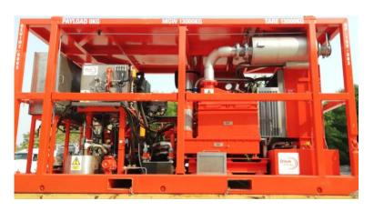
The unit has been designed to meet the requirements of ATEX, PED and the Machinery Safety Directive and the structural design reviewed by DNV to 2.7-1 and EN12079.
