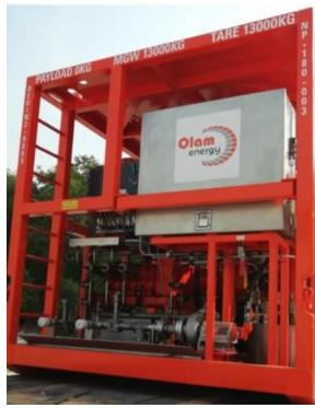
The skid has a four point lift incorporating fork lift pockets and has been approved by DNV.
